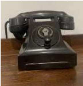
Hand crank desk phone with separate subscriber box (not shown) that was mounted on the wall near the phone with the ring bells and dry cell batteries.
